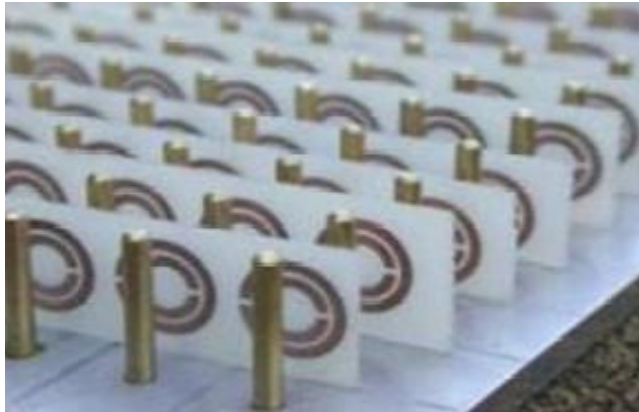
Fig (3): composite of thin wire and SRRs
